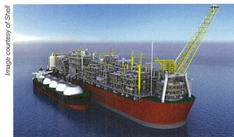
The Shell Prelude FLNG concept requires the world's largest ship; in comparison, multiple nitrogen cycle liquefaction trains can be installed on a ship the size of the LNG carrier next to the Prelude vessel
